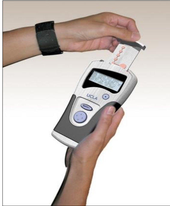
Figure 12 UCLA OFNASET® salivary sensor for oral cancer detection (19)
