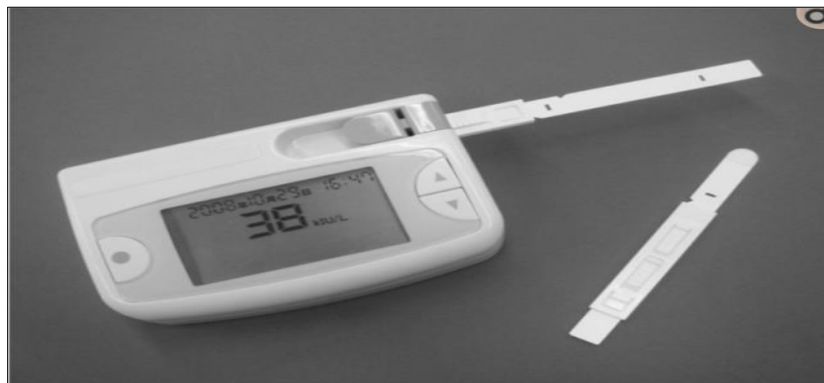
Figure 13 Portable sAA biosensor comprising a handheld reader and a disposable collection strip. (78)
