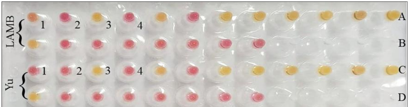
Figure 1 Illustrative RT-LAMP results for 20 samples using Lamb [8] (A and B lines) and Yu [9] (C and D lines) set of primers. The colors indicate Negative (rose) and positive (yellow) diagnostics for the presence of the SARS-CoV-2 virus. Sample #1 has divergent results between the primer sets, meanwhile, sample #4 (lines A and C) has a distinct result from RT-qPCR (supposed to be positive)
