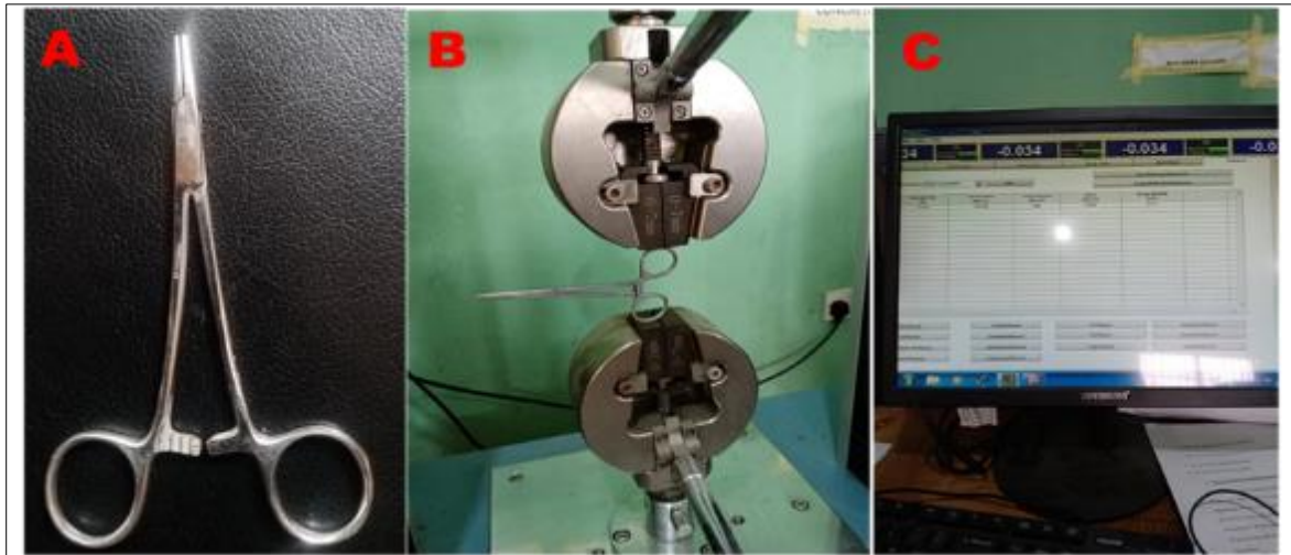
Figure 1 (A) haemostatic forceps, (B) determination of compressive force of forceps using Universal Testing Machine and (C) digital recording of the compressive force
