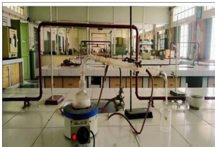
Figure 3 Distillation process for extraction of oil
